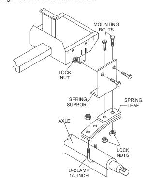
Figure 30. Suspension Components
